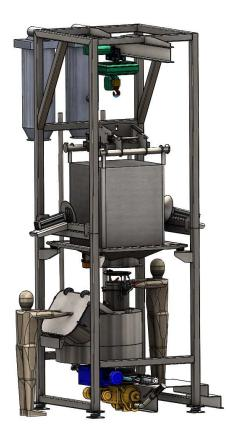
This station allows the big bag and sac emptying independently in a same hopper. This hopper is equipped with a flat-bottom extractor avoiding any phenomenon of bridging, while eliminating the clods of product.
