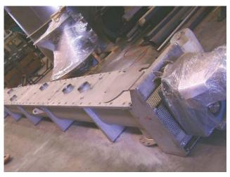
Installation of an Archimedean screw in the plastic industry
